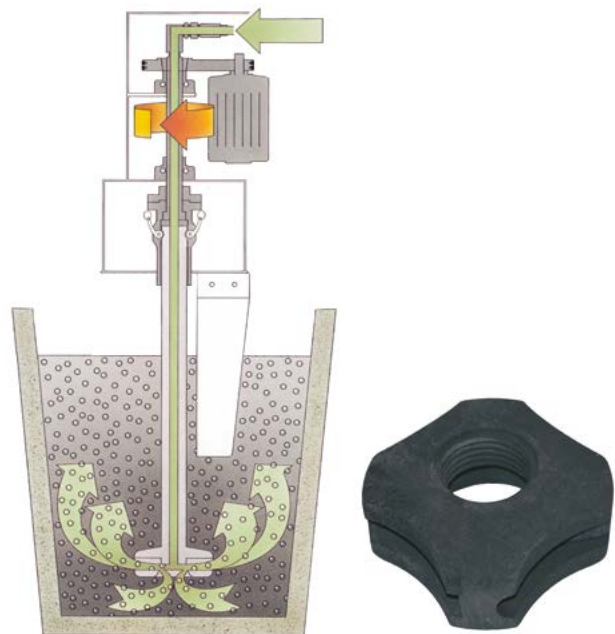
Figure 5: Effective degassing process using a Foseco Degassing Unit (left) and the patented impeller rotor (right)
